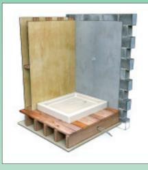
Timber joist shrinkage is common in new buildings causing the joint between the ledge & wall to expand
