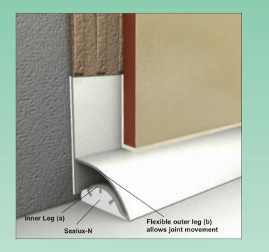
TRIMLUX combines a flexible pvc strip with Sealux-N silicone. The Sealux-N laid in the strip fuses with the Sealux-N laid on the ledge to form a watertight seal over the joint between the wall and the ledge.
