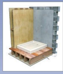
Shower trays not resting solidly on floors often rock causing the wall & ledge joint to expand
