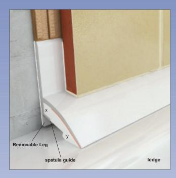
SEALUX combines a rigid pvc strip with Sealux-N silicone. To install Sealux the strip is filled with Sealux-N silicone and planted over the joint.
