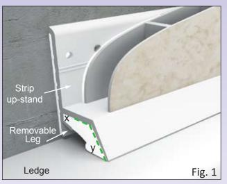
Cladseal combines a rigid pvc strip with Sealux-N silicone. Each strip has a green tape (green dotted line) applied to the inside face. This is a silicone bond breaker that prevents the silicone bonding to this part of the strip.
