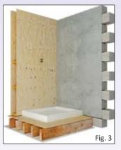
Timber joist shrinkage is common in new buildings causing the joint between the ledge & wall to expand. Semi-rigid acrylic baths and shower trays deflect when loaded with water and occupant causing the joint between the ledge and wall to expand.
