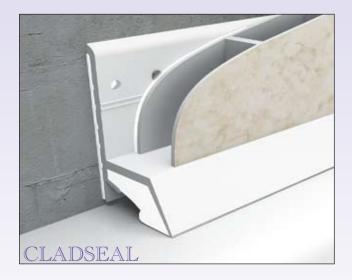
The sealant is concealed and protected inside the trim while a silicone bond-breaker tape releases the sealant off the trim for flexibility.
